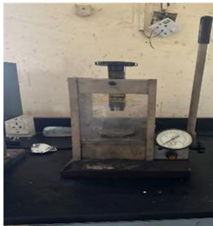
Fig. 1. Manual press machine used for compressive strength.
