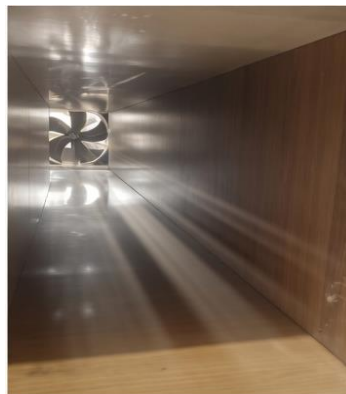
Fig. 3. Scheme of a wind tunnel with the axial fan at the outlet side.
