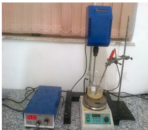
Fig. 3. Mixing ethanol with NaOH.
