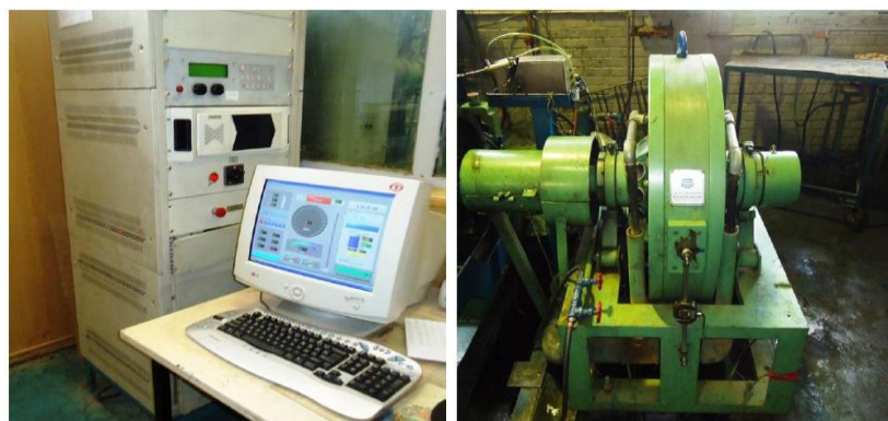
Fig. 6. Dynamometer, equipment control room and data acquisition.
